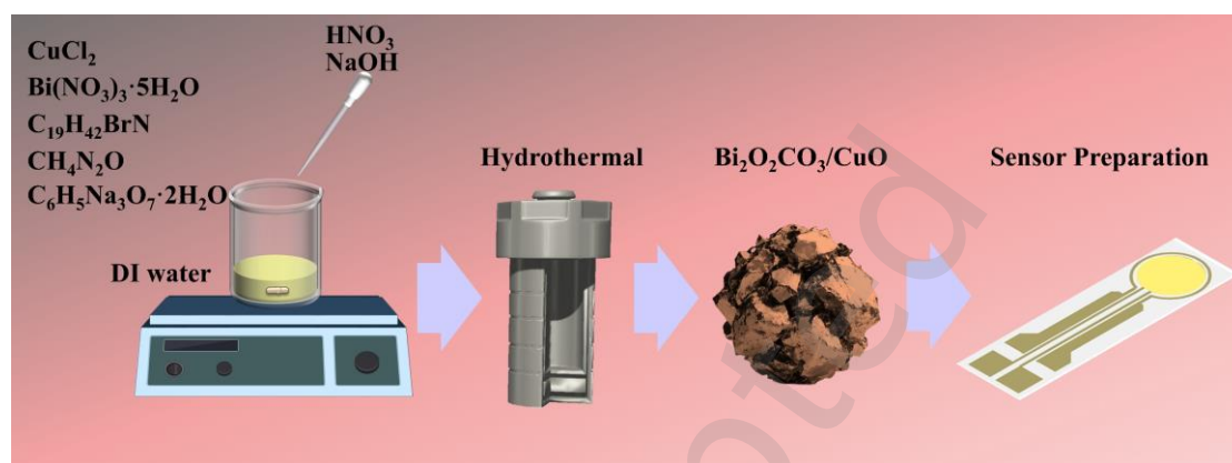
Fig. 1. Schematic illustrations of the fabrication process of \text{Cux-BC} microstructure.
